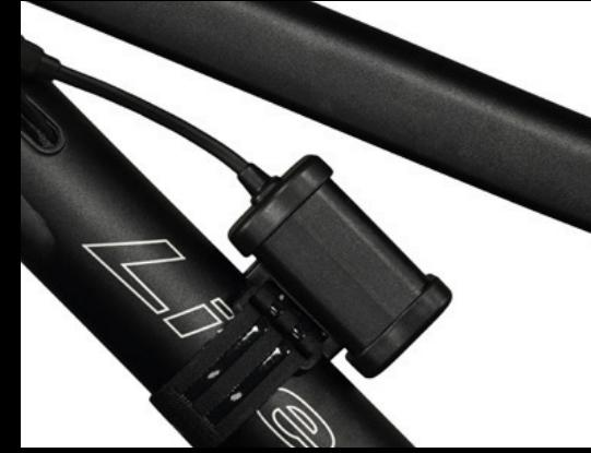
**Battery type:** The hardcase battery is mounted with a velcro as shown here. So called Smartcore batteries also come with a capacity indicator as explained on the next page.
